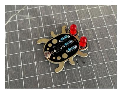
Hint - the transistor and the LED orientation is important and their outline is drawn on the PCB, simply match the flat parts and it will be oriented correctly.
