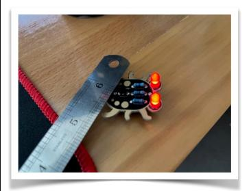
A very simple learn to solder kit that you can put together in minutes. Once put together and a battery inserted, the weevil will stay in the off state if the lights are on. Once lights go out however, it's red eyes will light up.
