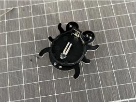
6. Insert a CR2032 coin battery cell into the battery holder.
