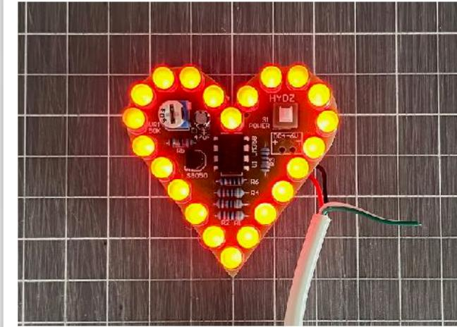
A moderate level learn to solder kit that includes an IC as well as standard components. The LEDs are red and have a 'breathing' light up effect.
