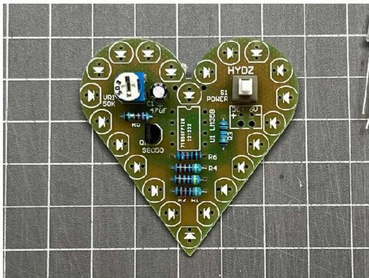
Hint - the capacitor orientation is important, make sure the stripe side of the capacitor lines up with the filled in part of the capacitor symbol side on the PCB. Alternatively look for the + sign on the PCB and align the side of the capacitor without the stripe to it.
