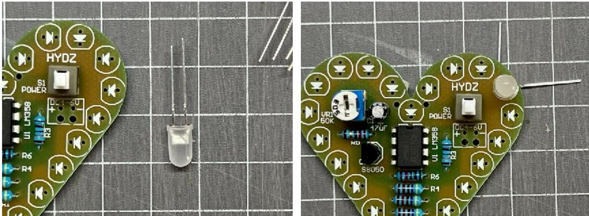
Hint - LEDs must be oriented correctly. The short leg is the side that has the flat edge at the base of the LED. Line up the short leg with the side of the LED symbol that also has a flat edge.
