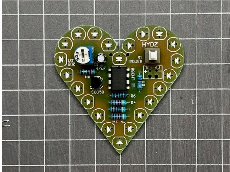
Hint - The notch on the IC must align with the notch on the IC symbol on the PCB.
