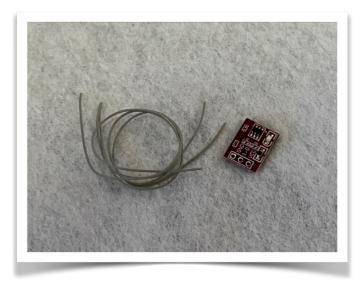
A touch module works just like a momentary button and can be placed under plastic parts to trigger and switch PCBs on/off.
