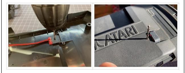
**5.** Secure the PCB. Push the screw through the outside of the case, through the PCB and the 3D printed cover, so that it's visible on the inside of the case. Tighten the nut on the screw. You can use a 2.5mm Allen key or just tighten it as much as you can using your hands. Don't tighten too hard to avoid cracking the plastic.
