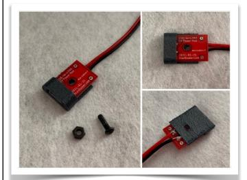
This kit adds a micro-USB power socket to the back of your Lynx and bypasses the 9V circuit to power your Lynx directly from USB.
