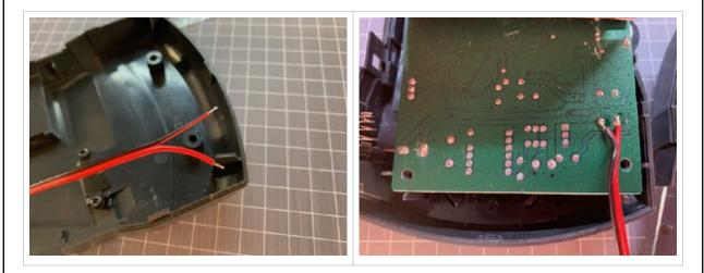
**7.** Test and re-assemble the Lynx. Use a USB power supply or a USB battery bank with a micro-USB connector to test your mod. You will need to have at least a 1A USB power source. If you're using a McWill LCD modded Lynx, you will need to have more than 1A to avoid the power LED on the Lynx from flashing. Plug in a micro-USB cable into your Lynx and USB power source, your Lynx will power on immediately. There is no on/off functionality when using this mod as mentioned earlier.
