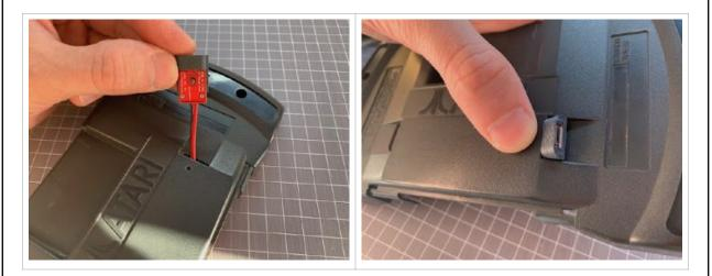
**4.** Drill a screw hole. Make sure the PCB is flat against the inside of the Lynx shell (you may need to hold it). Using a 2.5mm drill bit, drill out a hole in the Lynx case that lines up with the screw hole in the PCB and 3D printed cover. Clean up any plastic shavings left over after drilling the hole.
