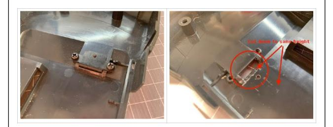
**3.** Insert the USB socket. Once the strap loop space is cleared out, insert the PCB with the USB socket as pictured. You may need to cut out more on the sides around where the strap loop was. The PCB and 3D printed cover should slide in easily when you get the cutout right.
