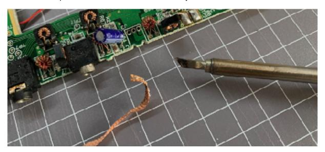
**4.** Solder in the new socket. Push the new socket in, use some Blu-Tac (or similar) to hold it in place, then solder it's legs into the motherboard. Trim the legs if required. Then using some IPA clean any remaining flux residue.
