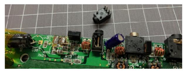
**3.** Desolder the power socket. Flip the Lynx motherboard around to the bottom side and either using a desolder gun or desoldering braid, remove the solder around the three pins that secure the power socket. Be careful to not lift any traces.
