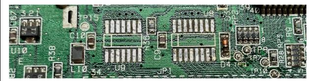
**6.** Solder in the new ICs, making sure that the stripe aligns to the stripe drawn on the motherboard (or where the old ICs had a notch).
