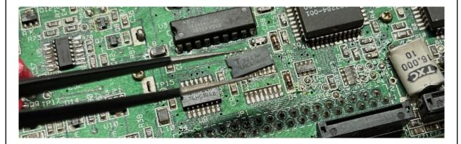
5. Once the ICs are removed, clean up the motherboard pads with solder braid.
