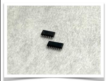
If your Lynx always shows the 'INSERT GAME' screen and can't read any cartridge, its I/O ICs may be bad. This is a replacement kit for the two ICs responsible for reading data off the cart. Our Atari Lynx repair kits use only premium components.
