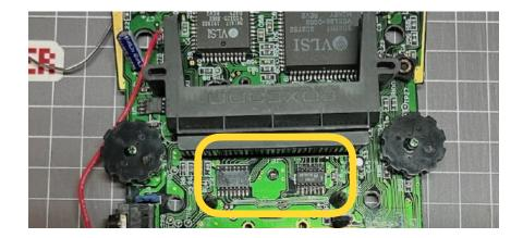
**4.** Desolder the original ICs. This can be done with either a soldering iron and desoldering braid or with a hot air gun for SMD work. Either way, use lots of flux. If you're using a soldering iron, you may want to snip off the legs on the ICs first using side cutters.
