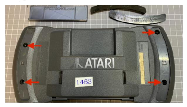
**Step 3** - There are some plastic 'clips' on the two parts of the Lynx 2 case that hold the case together even without the need for screws. These are not usually very tightly bound. To separate the two halves of the case, it is easiest to start by uncoupling the clips around the battery compartment and moving around to the sides next. With a little bit of twisting, the two halves should come apart without the need to wedge a screwdriver between them.
