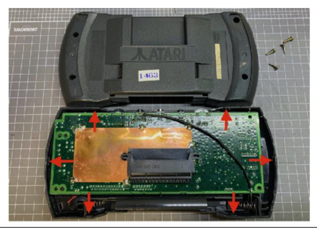
**Step 4** - Remove the single screw that is holding the battery compartment in place. The compartment plastic can then be lifted out, you will need to lift the motherboard up slightly to give enough room for the spring side of the battery terminal to clear enough space.
