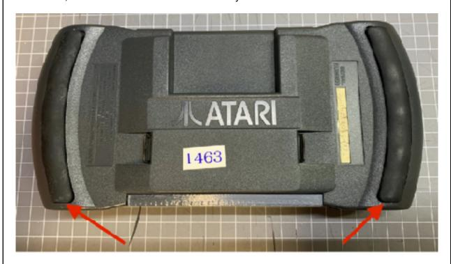
**Step 2** - Take out the battery cover (we have a 3D printed replacement on our model Lynx) and then using a Phillips screwdriver, remove the four screws that were hidden under the rubber grips.
