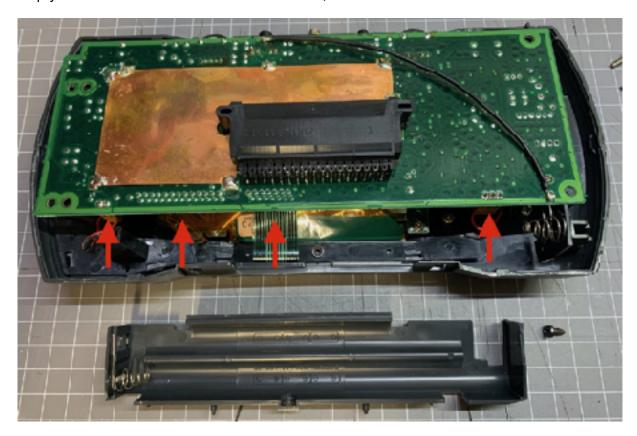
**Step 6** - The screen and controller assembly are held in place by four and six screws, respectively. These are of different size. Unscrew these.
